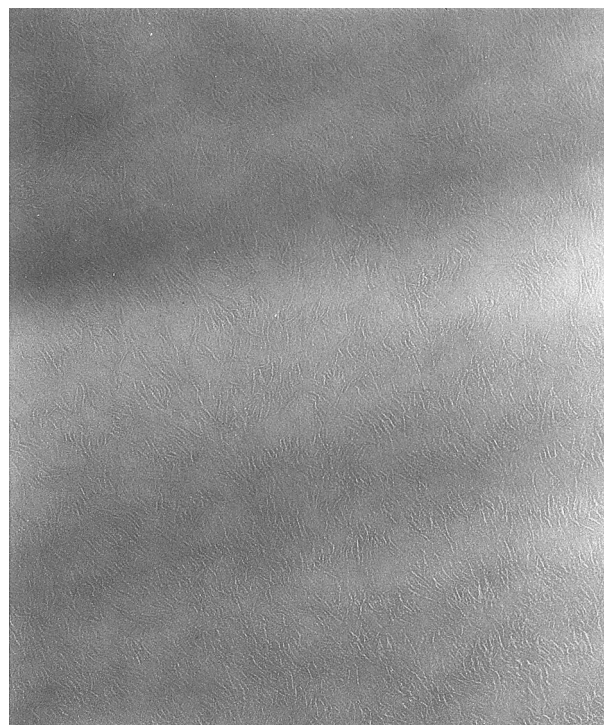
Fig. 11. TEM for an ethylene–hexene copolymer without long-chain branches. M_w = 68,000 g/mol; 1.14 mol% branch points.
