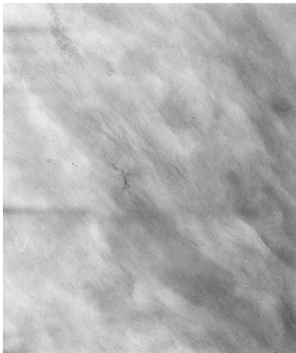
Fig. 12. TEM for an ethylene–octene copolymer without long-chain branches. M_w = 79,000 g/mol; 1.4 mol% branch points.
